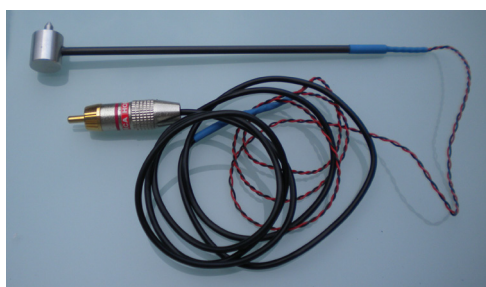
SMIA Low Mass pulsehammer with integrated force sensor
